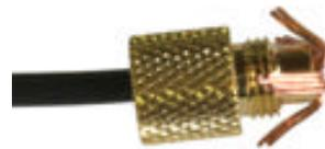
**Step 4:** Clip the strands, if necessary, so that none of them are long enough to reach the threads.
